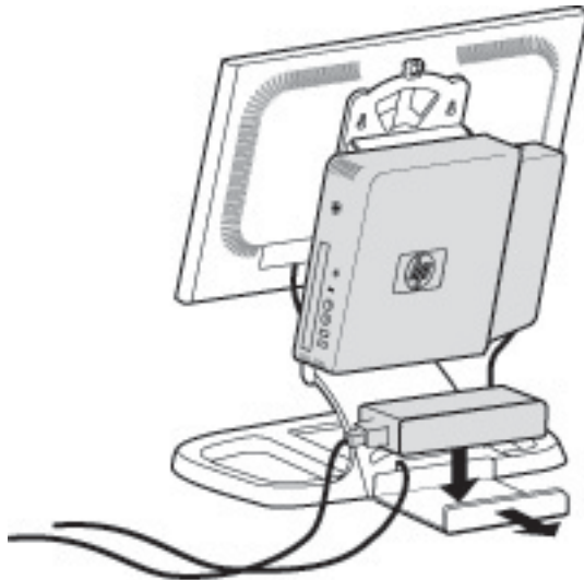
Figure 3-11 Installing the Power Supply
