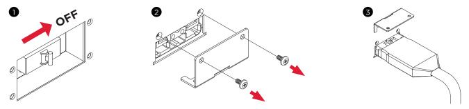
Step 4: Rotate the battery cable retention bracket and tighten the two screws to fix battery cable.
