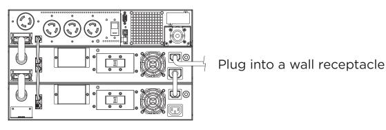
Step 1: Turn off the DC breaker on the EBM.
