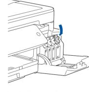
Push down on the cap of the ink tank to close it tightly. Repeat step 6 for the three other ink tanks.
