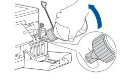
Remove the tip of the ink bottle. Insert the nozzle of the ink bottle firmly so that the ink does not spill. Fill the ink tank by gently squeezing the bottle as shown. Empty the entire bottle into the ink tank.
