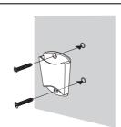
2. Stick to the wall and fix it with screws.
