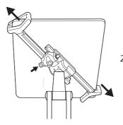
2. Press and hold on the release button to unlock the frame.
