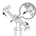
1. Press and hold on the release button to unlock the frame.
