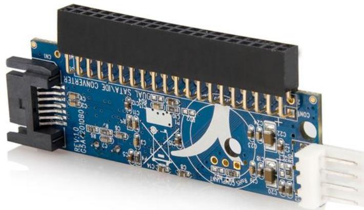
This IDE to SATA adapter converts a 40-pin IDE connector to a SATA connector, allowing you to connect a 2.5in or 3.5in SATA (SATA, SATA II/SATA 300) drive to the motherboard in place of an IDE drive.
