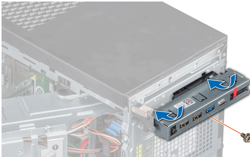
Figure 53. Installing the control panel
