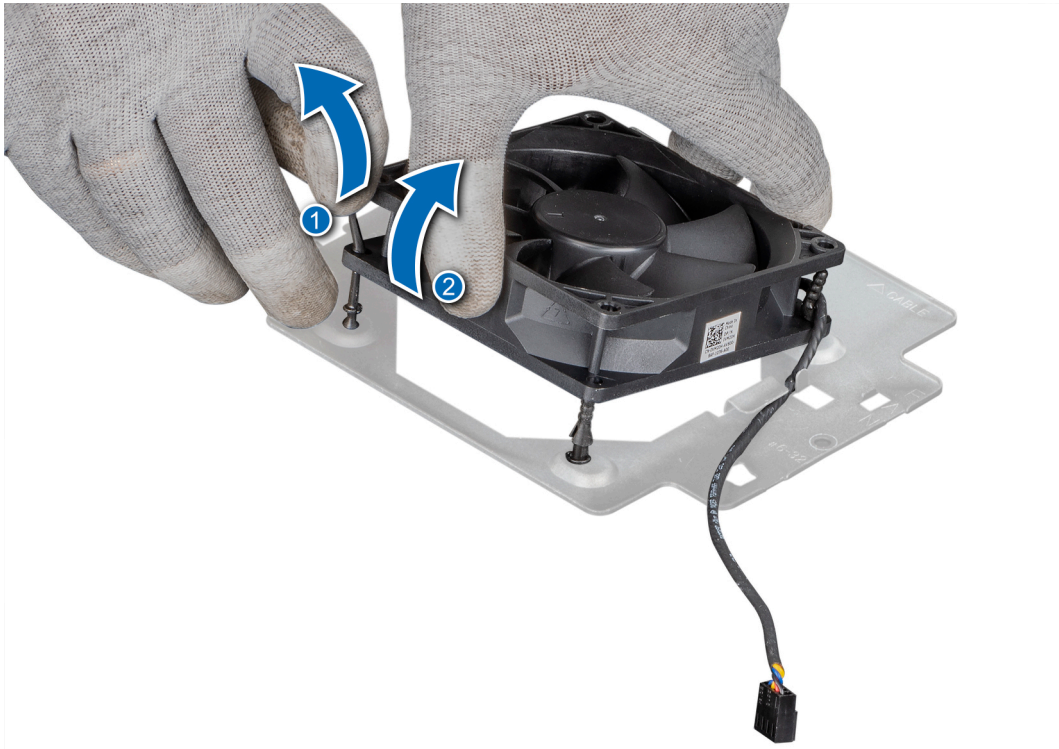
Figure 38. Removing the System fan
