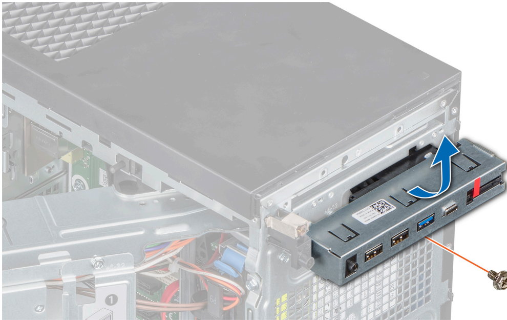
Figure 52. Removal of the control panel
