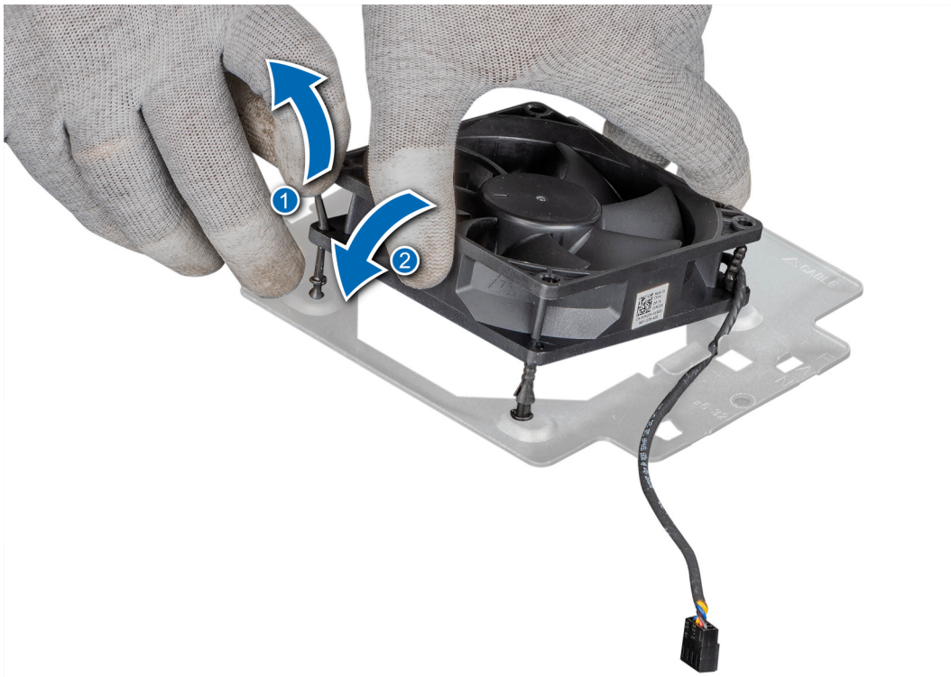
Figure 39. Installing system fan
