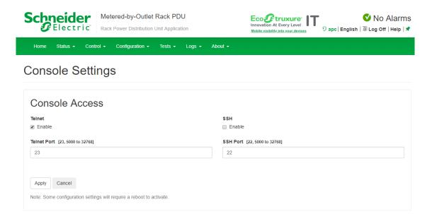
**Telnet for basic access:** Telnet provides the basic security of authentication by user name and password, but not the high-security benefits of encryption. Telnet is disabled by default.
