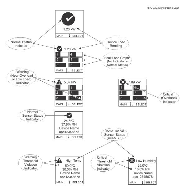
**NOTE 1:** The simplified LCD pages will show device load alarms only when no banks are present OR bank load alarms only when banks are present. Phase and Outlet alarms and warnings will NOT be displayed.
