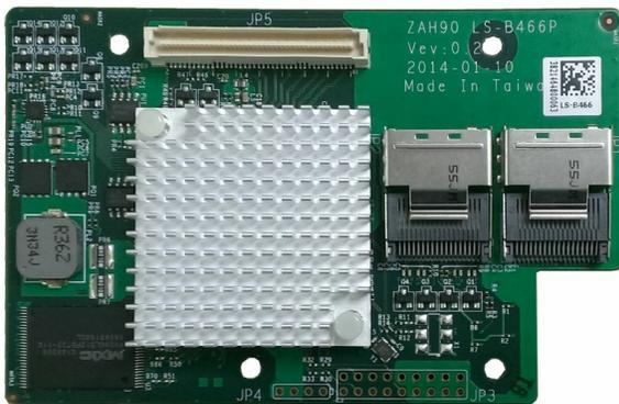
Figure 8. H701-L RAID adapter (air baffle removed)
