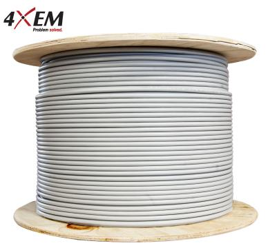
4XEM CAT6 exceeds requirements of TIA/EIA-568-B.2-1. It is ideal for high-end solutions such as Gigabit Ethernet, 1.2Gbps ATM, and broadband video. This Cable consists of eight solid 24AWG wires and a separator to separate four pairs. 1000 ft Roll of Cat6 Cable 24AWG, 0.5mm CCA White
