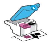
**e.** Check if there is a plug on top of the printhead or plastic tape on the printhead contacts. If there is, remove the plug from top of the printhead and the plastic tape from contacts.
