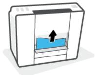
Close the cleanout door. Gently push the door towards the printer until both latches snap into place.
