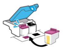
**g.** Close the printhead latch. Make sure the printhead latch is properly closed to avoid problems such as carriage jams.
