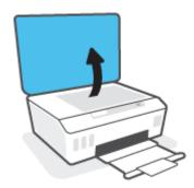
Clean the scanner glass and lid backing by using a soft, lint-free cloth that has been sprayed with a mild glass cleaner.
