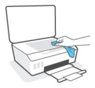
**CAUTION:** Use only glass cleaner to clean the scanner glass. Avoid cleaners that contain abrasives, acetone, benzene, and carbon tetrachloride, all of which can damage the scanner glass. Avoid isopropyl alcohol because it can leave streaks on the scanner glass.
