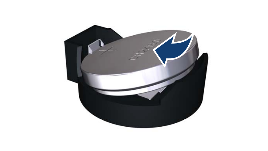
Figure 86: Installing the CMOS battery
