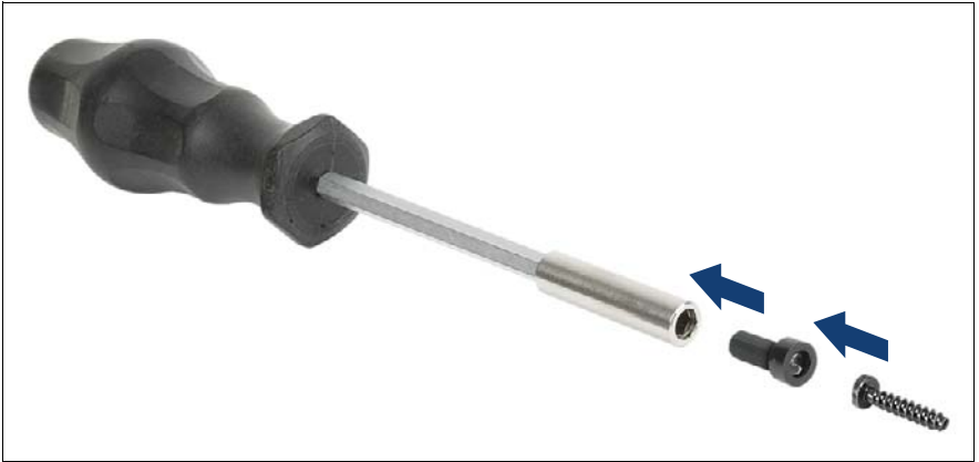
Figure 97: TPM bit insert
