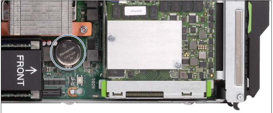
Figure 84: Location of the CMOS battery on the system board D3142 (see circle)
