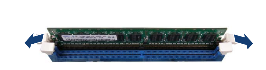
Figure 60: Opening the securing clips
