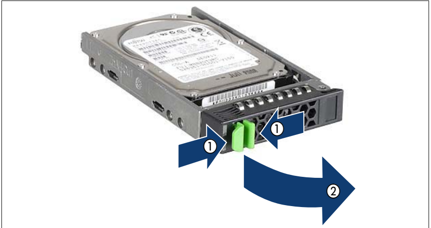
Figure 17: Unlocking the 2.5-inch HDD/SSD module
