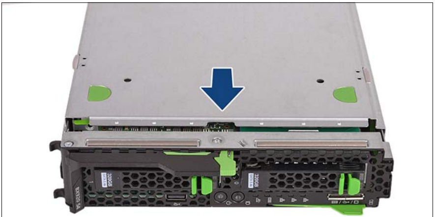
Figure 10: Closing the server blade
