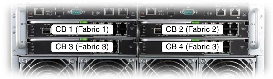
Figure 34: Connection blade slots (BX400 S1 system unit)
