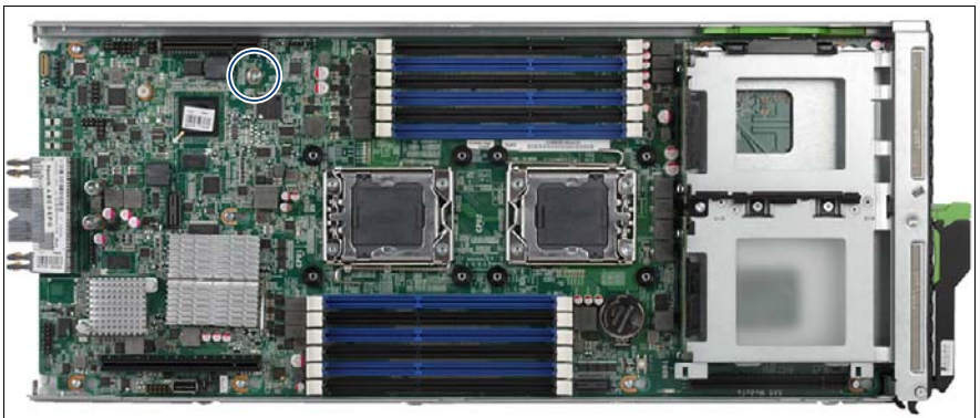
Figure 104: Detaching the system board (A)
