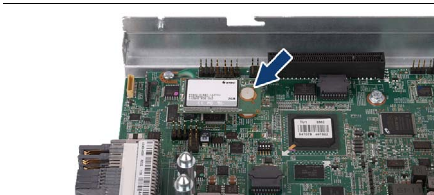
Figure 89: Installing the UFM
