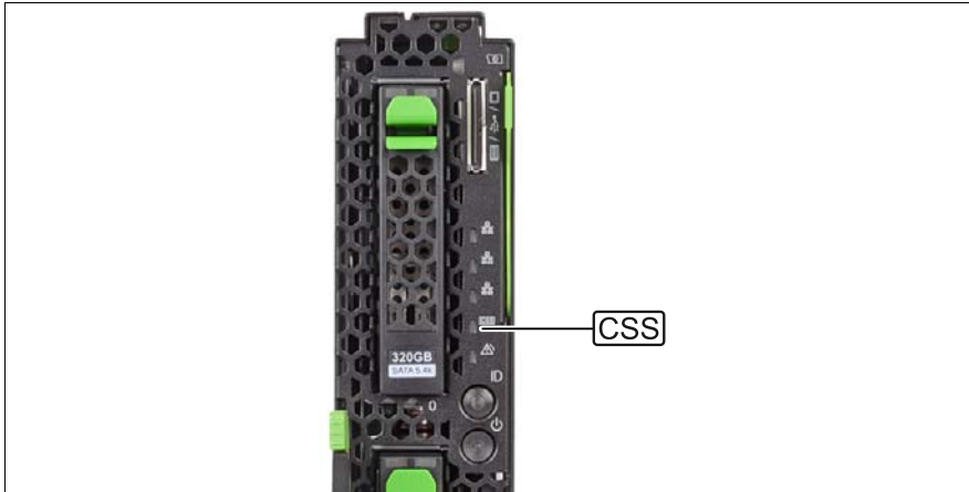
Figure 5: CSS error indicator in front panel
