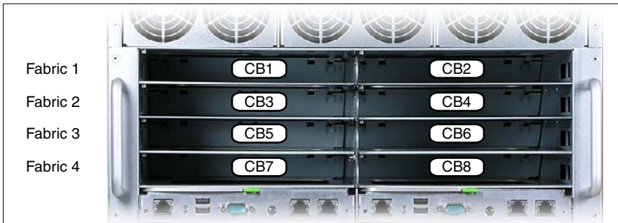
Figure 33: Connection blade slots
