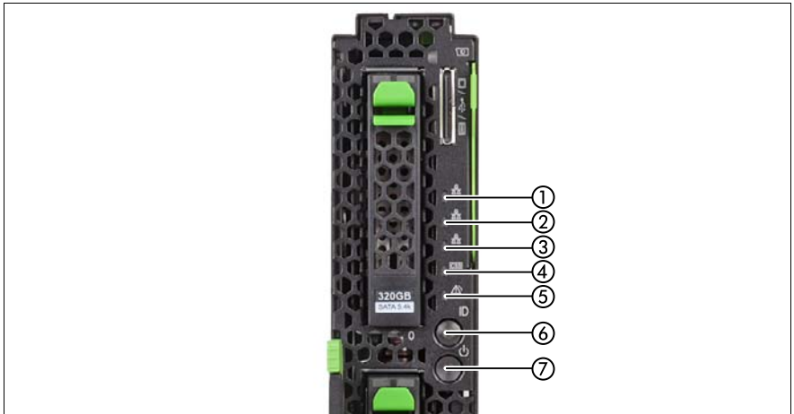
Figure 114: I/O panel indicators
