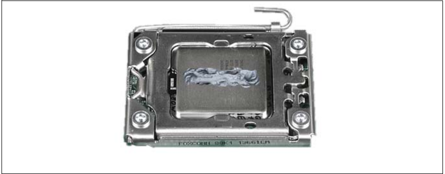
Figure 83: Applying thermal paste
