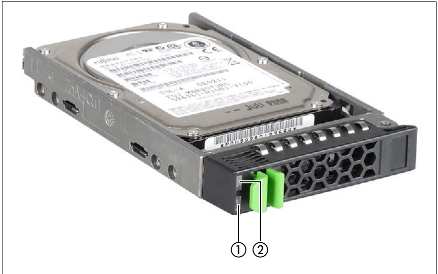
Figure 115: Indicators on the 2.5-inch HDD module
