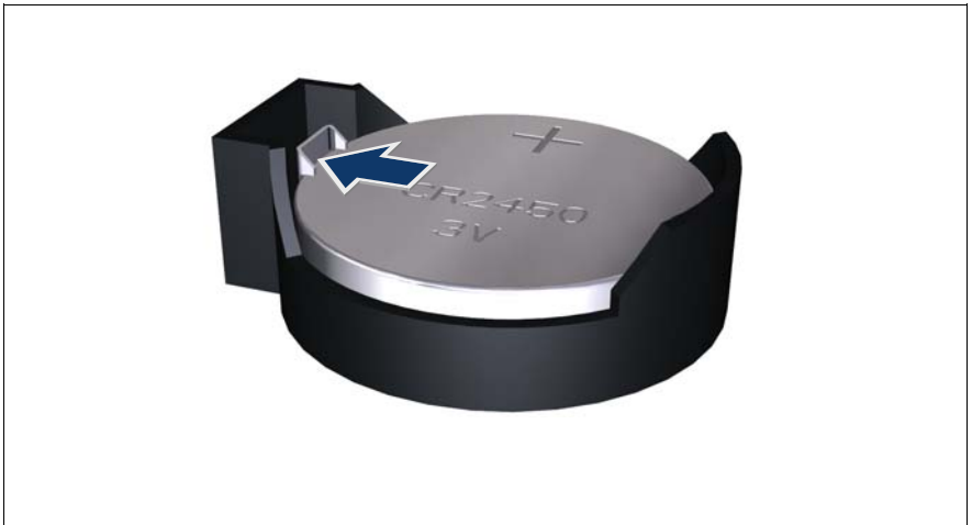
Figure 85: Replacing the CMOS battery
