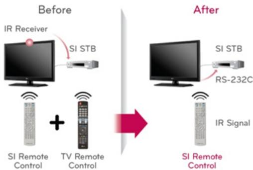
The IR Out enables customised set-top boxes to receive IR signals via the LG TV Signage with the STB remote control. It provides added convenience with simpler connection and allows easy management using a single remote control.
