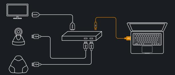
It's as simple as it is ingenious, wouldn't you say? This is how the components of the video packages fit together, with the Konftel OCC Hub making the solution a breeze to set up and use. As the name suggest, the Konftel OCC Hub sits at the heart of the video collaboration solution, offering One Cable Connection to the conference camera, speakerphone and screen.
