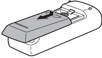
2. See the instructions in the compartment and put in the supplied batteries (R-6 ("AA" size) x 2) with their plus (+) and minus (-) sides oriented correctly.
