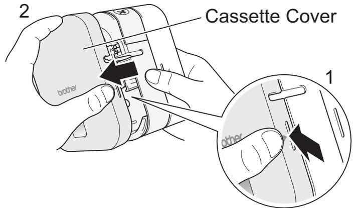
2. Insert the Tape Cassette following the drawing marked inside the case. Confirm that the tape is aimed at the green Tape Outlet and gently press the Tape Cassette into your machine until it locks into place.
