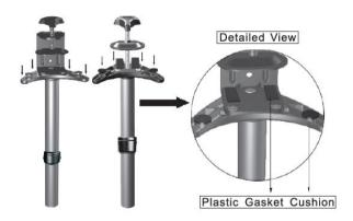
3. **Desk Clamp:** Place the Desk Clamp **(3)** opening around the edge of your desktop in your desired location and tighten by hand to secure. Ensure that the Desk Clamp is making full contact with the desk surface.
