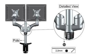
3. Place the Cover (11) over the mounting post and insert 1 x M6x12mm Phillips Screw (16) with 1 x Plastic Washer (15). Tighten using a Phillips screwdriver.
