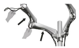
3. Use the Cable Clip (14) to secure the display cables to the pole.
