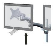
**Note:** For all adjustments outlined below, turning the screw clockwise will increase the resistance, while turning the screw counter-clockwise will decrease resistance.
