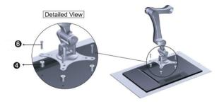
3. Using a Phillips screwdriver, tighten the screws until the bracket is firmly attached to the back of the display.
