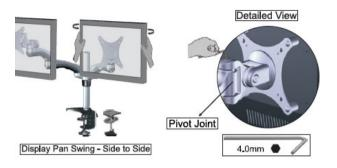
To increase / decrease the swivel resistance on either of the elbow joints of the articulating LCD Arms, adjust the set screws indicated below, using the 2.5mm Allen Wrench (10)
