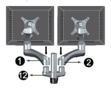
2. Tighten the set screw using the 2.5mm Allen Wrench (10).
