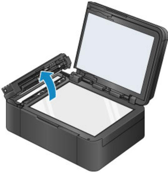
3. With the clean cloth, wipe off any paper dust from the inside of the document feeder cover (A).
