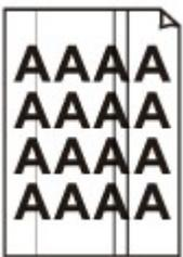
**Check7** Check that the original is loaded correctly on the platen glass or in the ADF.
