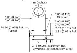
0.03 (0.001) Minimum Ref. (applies to top edge of gasket or edge of crimp, whichever is higher)
