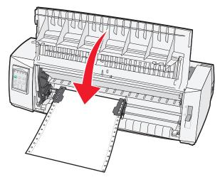
**13** Press **Start/Stop** to load the paper to Top-Of-Form, and then put the printer online.
