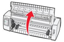
**4** Hold down the latching levers while you lift and pull out the tractor unit from the printer.
