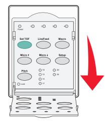
**5** Press any paper movement button (**Micro**  $\uparrow$ , **Micro**  $\downarrow$ , or **LineFeed**) to move the paper to the Top-Of-Form position.
