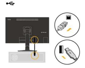
4. Connect one end of the USB 3.0 cable to the USB connector on the back of the computer, and the other end to the upstream USB connector on the monitor.
