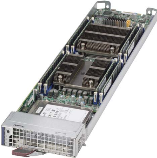
Figure 4-1. MBI-6128R-T2/T2X Blade Unit Front View
