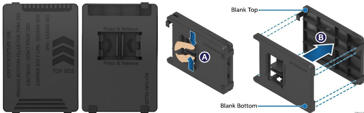
Figure 59. 2.5" Hot-Swap Drive Blank Top / Bottom and Attaching the Two
