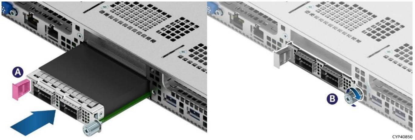
Figure 55. OCP* Adapter with Pull Tab Installation
