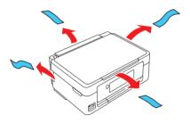
2 Lift up the scanner unit and remove all protective materials from inside the product.
