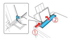
**Note:** Make sure you place the paper against the right side of the rear paper feed slot. Otherwise, the printer cannot detect the paper and the paper setup screen is not displayed on the control panel.
