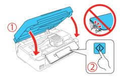
7 The printer starts charging the ink. Ink charging takes approximately 4 minutes. When you see a completion message on the printer's LCD screen, charging is complete.
