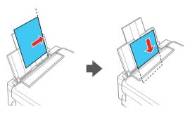
**5** Slide the edge guide against the paper, but not too tightly, and flip the feeder guard back.
