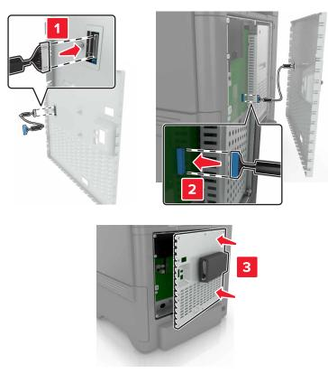
7 Reattach the controller board access cover.
