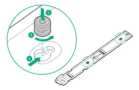
11. Install the rubber stoppers in the new locations to secure the PEM nuts in the M.2 riser.
