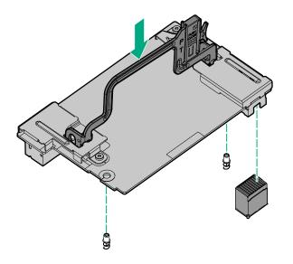
9. Close the storage controller handle to seat the storage controller on the connector.
