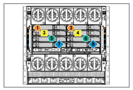
To support network connections for specific signals, install an interconnect module in the bay corresponding to the FlexibleLOM or mezzanine signals.
