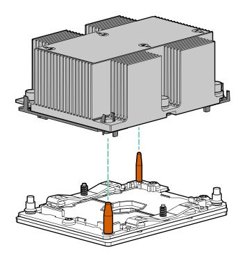
**9.** Using a T-30 Torx screwdriver, fully tighten each heatsink nut in the order indicated on the heatsink label (1 > 2 > 3 > 4) until it no longer turns.
