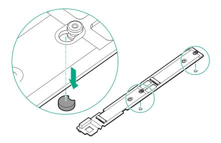
9. Remove the PEM nuts from the M.2 riser.
