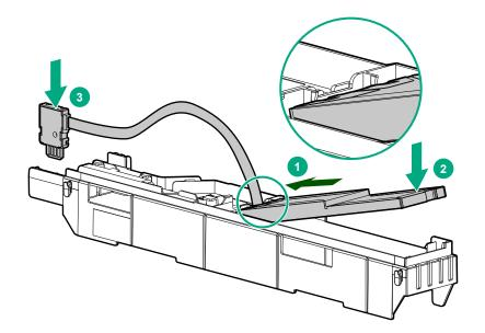
9. Route the cable on the right DIMM baffle.
