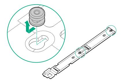
10. Install the PEM nuts in the new location on the M.2 riser.
