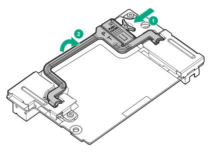
8. Align the storage controller with the alignment pins and lower it onto the connector.
