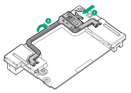
7. Remove the storage controller/NVMe pass-through board.
