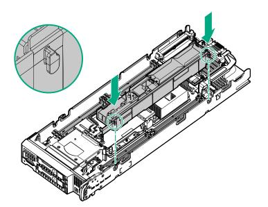
• DIMM baffle (left side)
