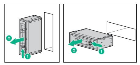
2. Remove the enclosure connector cover.
