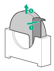
() **IMPORTANT:** Replacing the system board battery resets the system ROM to its default configuration. After replacing the battery, reconfigure the system through UEFI System Utilities.
