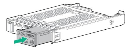
**3.** Install the SFF Flash Adapter by pushing firmly near the left-side adapter ejection handle until the latching spring engages in the drive bay.
