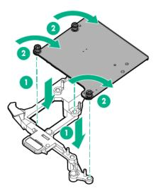
Align the mezzanine assembly with the guide pins on the system board, and then install the mezzanine assembly on the system board.
