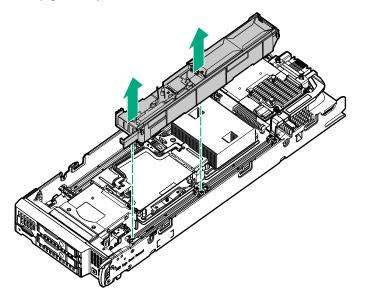
• DIMM baffle (left side)
