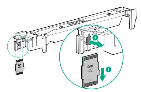
7. Remove the M.2 riser board from the left DIMM baffle.
