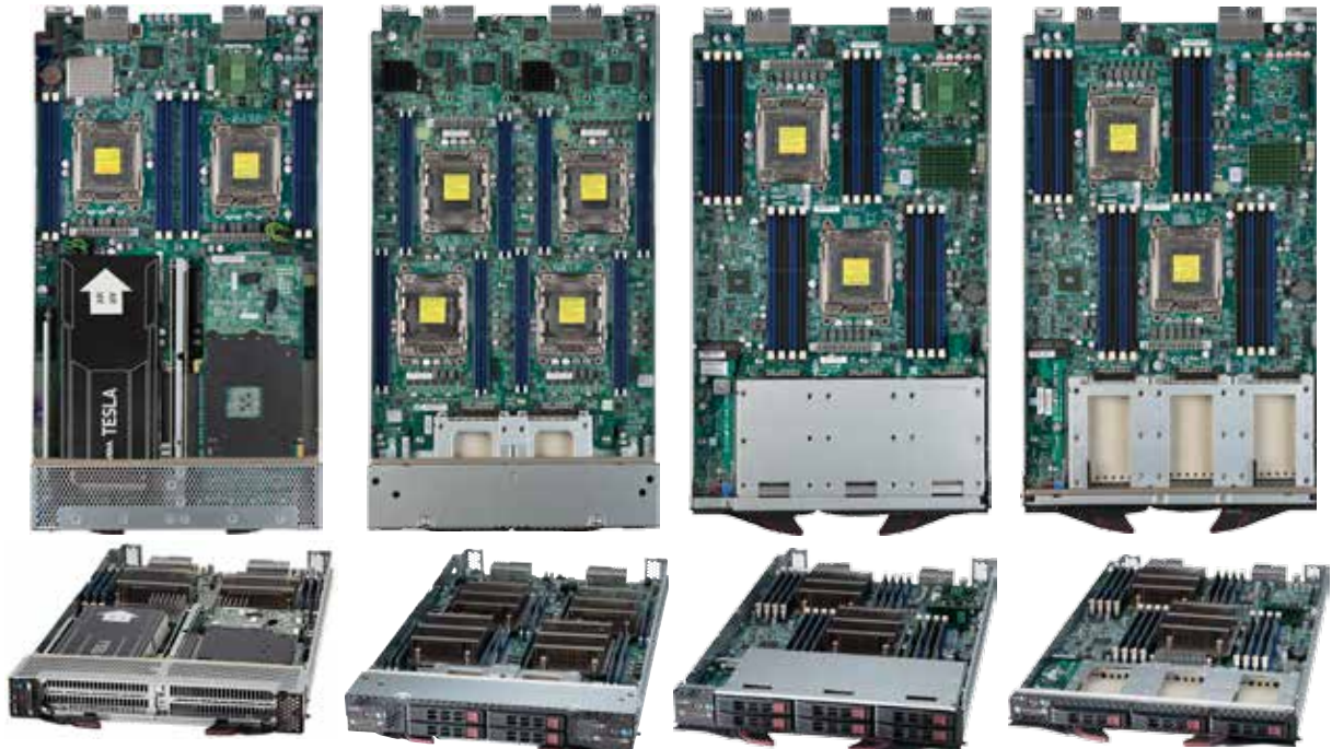
Sandy Bridge GPU/MIC SuperBlade® (2 CPUs + 2 GPU/MIC cards)
