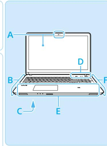
**F** USB port x 2 (Compliant with the USB 2.0 standard.)
