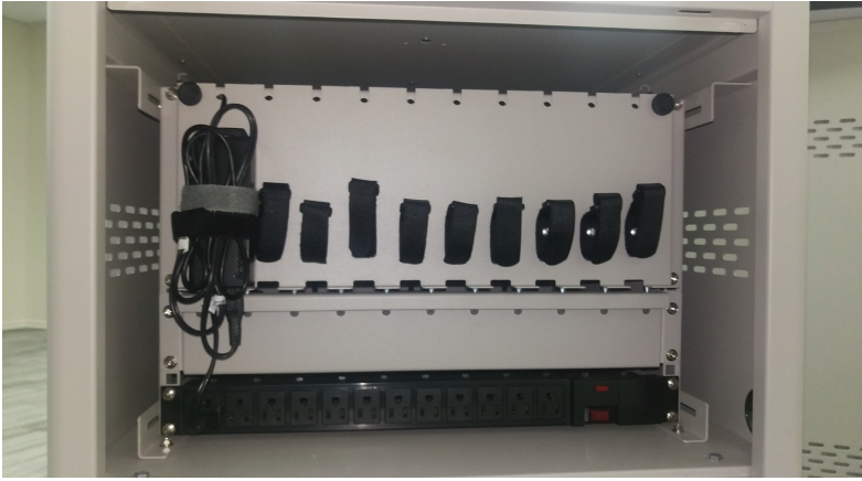
Figure 3-6. Fastening the power brick and routing the cable.
