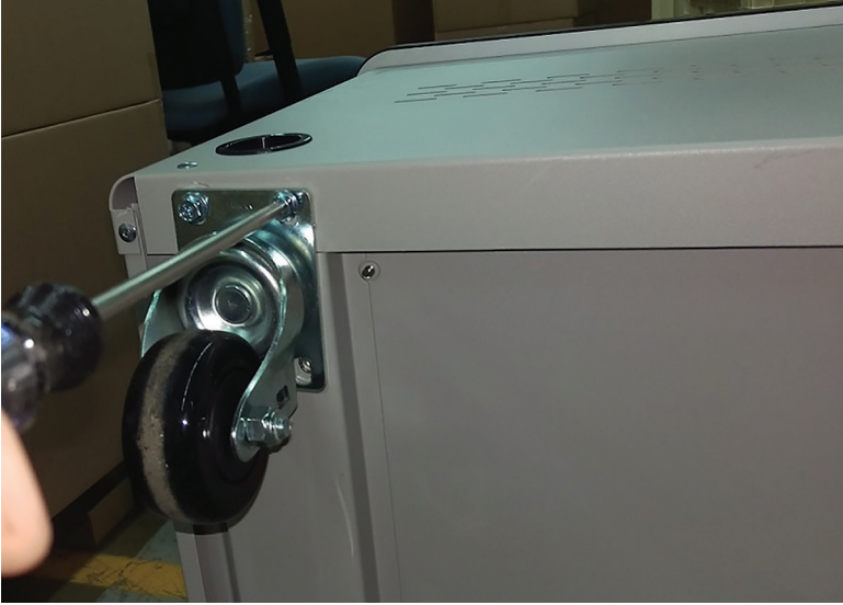
Figure 3-2. Attaching the Casters.
