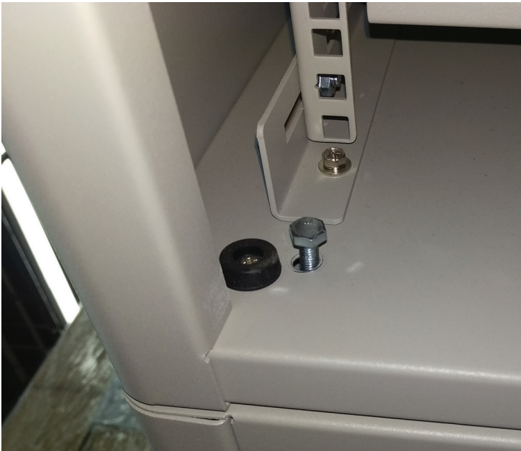
Figure 3-1. Attaching the Drawer.
