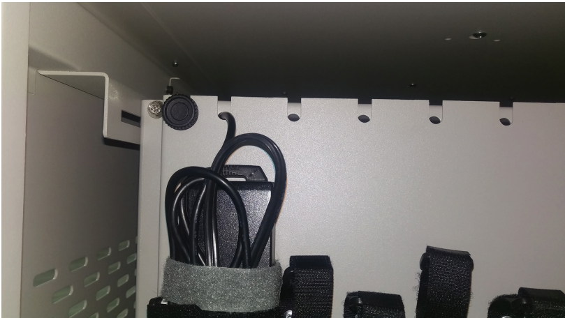
Figure 3-5. Attaching the power brick.
