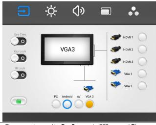
The users can keep pushing **Eye Care** on the OSD menu and **Classroom** under color temp. **Eye Care** and **Classroom** will be shown with the low blue light mode and the flicker free function. In **Eye Care** mode, the default value of **Brightness** and **Contrast** both are 50 and the default value of Backlight is 10.
