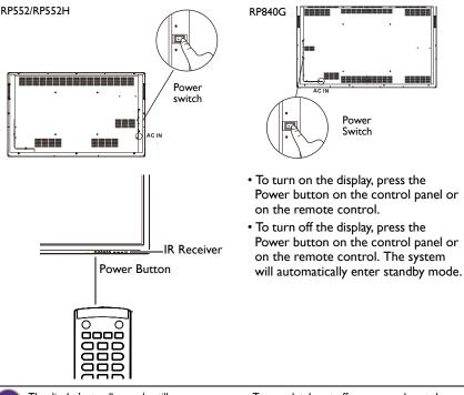
The display's standby mode still consumes power. To completely cut off power supply, set the Power switch to OFF  $(\mathbf{O})$  and then disconnect the power cord from the power outlet.
