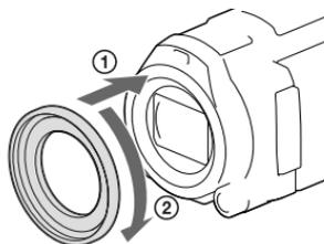
Align the Step Down Ring with the camcorder properly (①), then turn it in the direction of the arrow until the Step Down Ring is locked in place (②).
