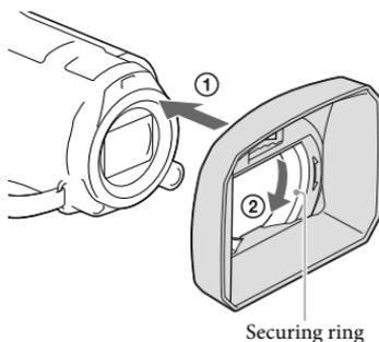
Align the lens hood with the camcorder properly (①), then turn the securing ring of the lens hood in the direction of the arrow (②).
