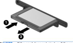
**NOTE:** If the card does not eject, pull the card out of the slot.
