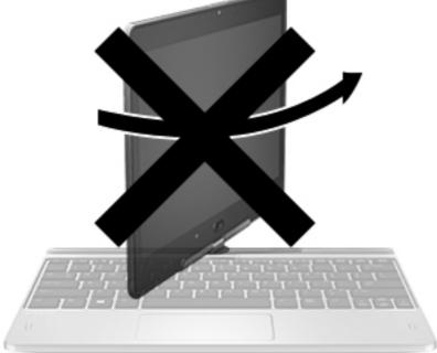
**CAUTION:** To prevent damage to the display hinges, , when in notebook configuration, do not rotate the display counterclockwise, and do not force the rotating action.
