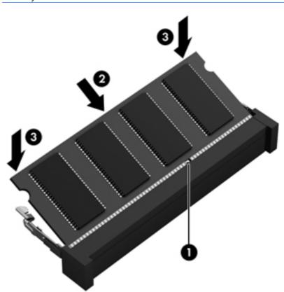
A CAUTION: To prevent damage to the memory module, be sure that you do not bend the memory module.
