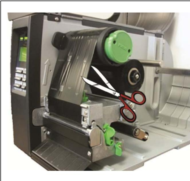
1. Break the ribbon between ribbon guide plate and the ribbon rewind spindle.
