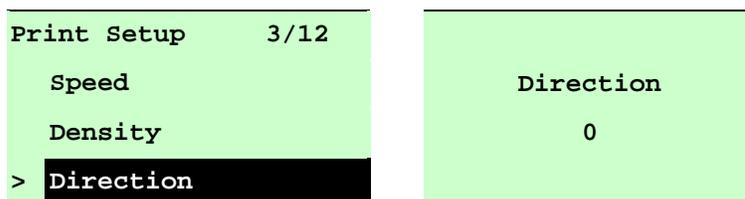
The direction setting value is either 1 or 0. Use this option to setup the printout direction. Printer default printout direction is DIRECTION 0.
