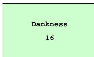
Use this option to setup printing darkness. The available setting is from 0 to 30, and the step is 1. Printer default density is 16. You may need to adjust your density based on selected media. Press **UP** and **DOWN** to increase/decrease the printing darkness. Press **SELECT** key to enable the setting. Press **MENU** key to cancel the setting and return to the previous menu.
