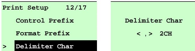
This option is used to set delimiter character. Press the **DOWN** button to move the cursor from left digit to right digit, and press the **UP** button to set the value from “0” to “9” or “A” to “F”. Press the **SELECT** button to set the value into printer. Press **MENU** key to cancel the setting and return to the previous menu.
