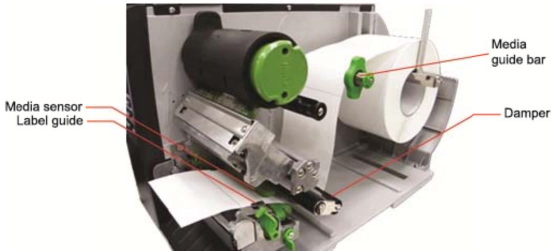
6. Unlock the media sensor lock lever to adjust the media sensor.
