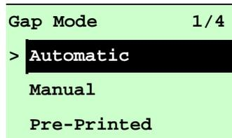
Press the **UP** and **DOWN** buttons to scroll the cursor to the media type and press the **SELECT** button to enter the sensor calibration mode.
