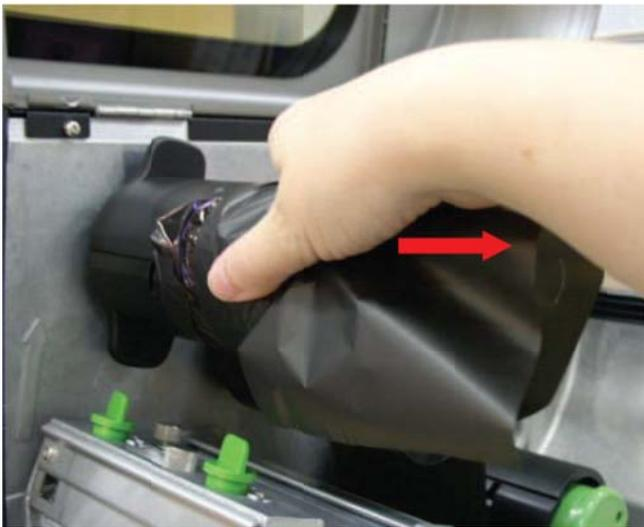
3. Then, slide off the ribbon from ribbon rewind spindle.
