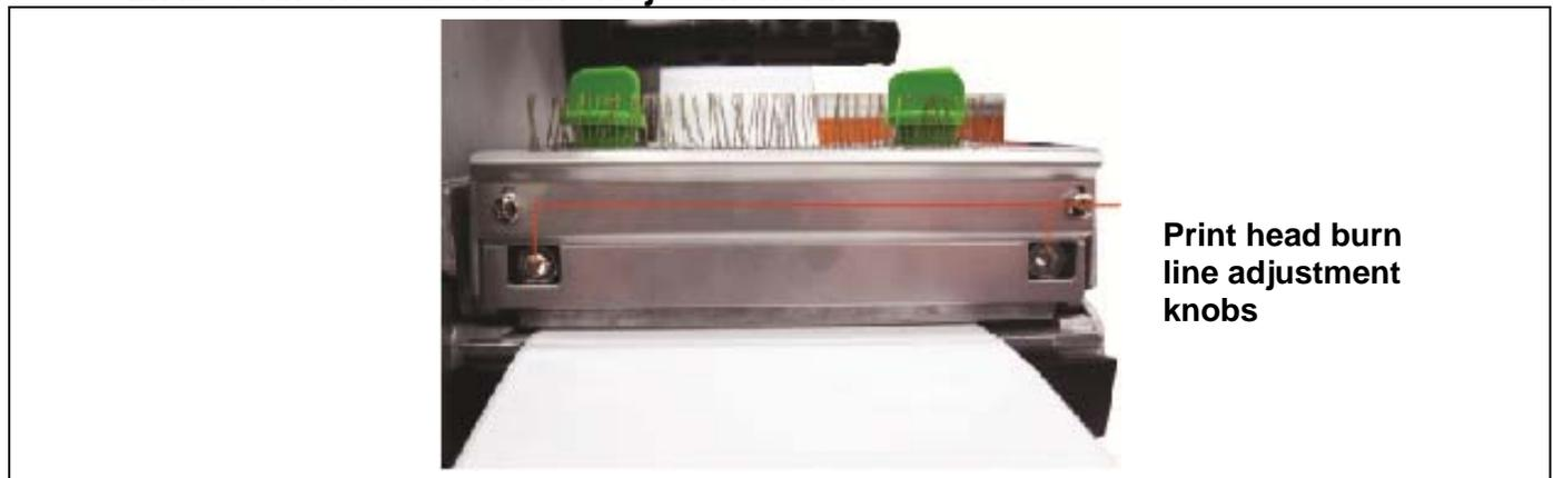
The print head burn line adjustment knobs are used to fine tune the print quality for different thickness of media. Turning the knobs adjusts the print head's burn line forward or backward as it relates to the platen roller.
