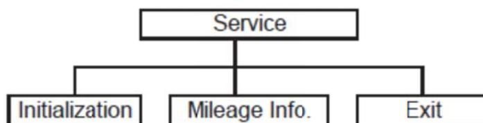
This feature is used to restore printer settings to defaults and display printer mileage information.
