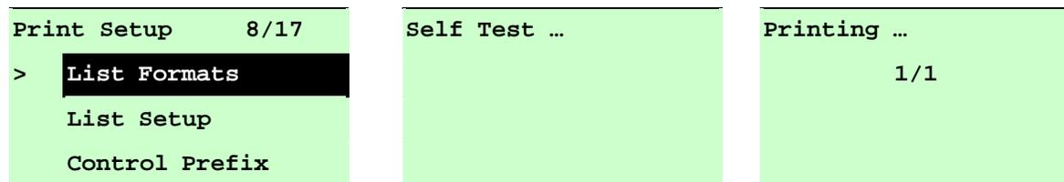
This feature is used to print current printer available formats list to the label. The formats are stored in the printer's DRAM, Flash or optional memory card. Press **SELECT** button to print the list.
