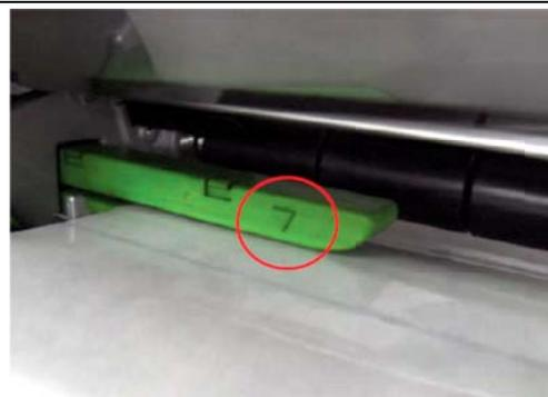
\* The sensor location is marked by a triangle mark
