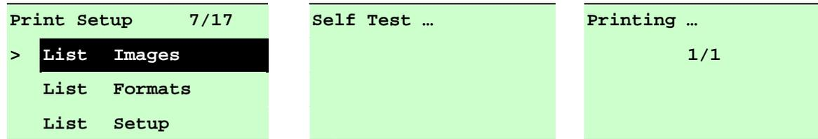
This feature is used to print current printer available images list to the label. The images are stored in the printer's DRAM, Flash or optional memory card. Press **SELECT** button to print the list.
