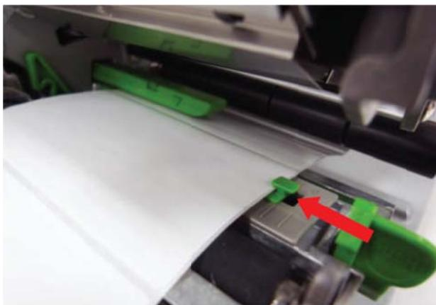
7. Adjust the label guide to fit the width of the label.
