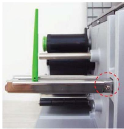
5. Pull label roll leading edge forward through the media guide bar, damper, media sensor and place the label leading edge onto the platen roller.
