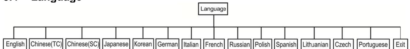
This option is used to setup the language on LCD display.
