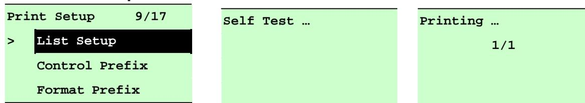
This feature is used to print current printer configuration to the label. Press **SELECT** button to print the list.
