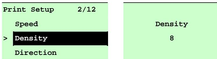
Use this option to setup printing darkness. The available setting is from 0 to 15, and the step is 1. Printer default density is 8. You may need to adjust your density based on selected media. Press **UP** and **DOWN** to increase/decrease the printing darkness. Press **SELECT** key to enable the setting. Press **MENU** key to cancel the setting and return to the previous menu.
