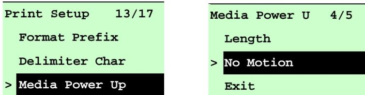
This option is used to set the action of the media when you turn on the printer. Printer default setting is No Motion. When entering this list, the mode on the right side of “>” icon is the current printer setting. Press **UP** and **DOWN** to select the different print mode and press **SELECT** button to enable the setting. Press **MENU** key to cancel the setting and return to the previous menu.
