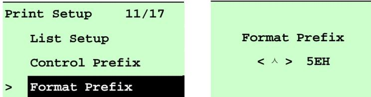
This option is used to set format prefix character. Press the **DOWN** button to move the cursor from left digit to right digit, and press the **UP** button to set the value from “0” to “9” or “A” to “F”. Press the **SELECT** button to set the value into printer. Press **MENU** key to cancel the setting and return to the previous menu.
