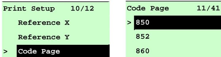
Use this option to set the code page of international character set. When entering this list, the code page on the right side of “>” icon is the current printer setting. Press the **UP** ⬆ and **DOWN** ⬇ to select the code page, and press the **SELECT** button to enable the setting. Press **MENU** key to cancel the setting and return to the previous menu.
