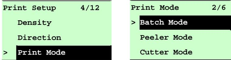
This option is used to set the print mode. Printer default setting is Batch Mode. When entering this list, the print mode on the right side of “>” icon is the current printer setting. Press **UP** and **DOWN** to select the different print mode and press **SELECT** button to enable the setting. Press **MENU** key to cancel the setting and return to the previous menu.
