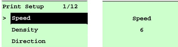
Use this option to setup print speed. The increment/decrement is 1 ips. Press **UP** key to raise the print speed, and press **DOWN** key to decrease print speed. Press **SELECT** key to set it into printer. Press **MENU** key to cancel the setting and return to the previous menu.
