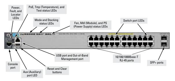
Figure 1-2. Front of the HP E3800-48G-PoE+-4SFP+ Switch
