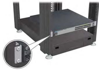
Figure 2-8. Mounting the switch in a rack
