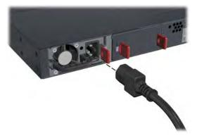
Figure 2-2. Connecting the power cord
