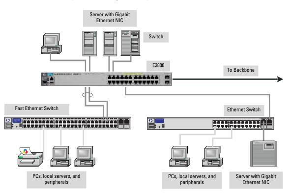
Figure 2-25. Example as a Segment Switch
