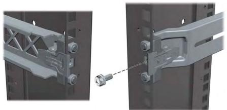
3. Installing the switch into the rails.
