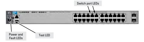
Figure 2-4.Example of an HP E3800-48-port PoE+ switch
