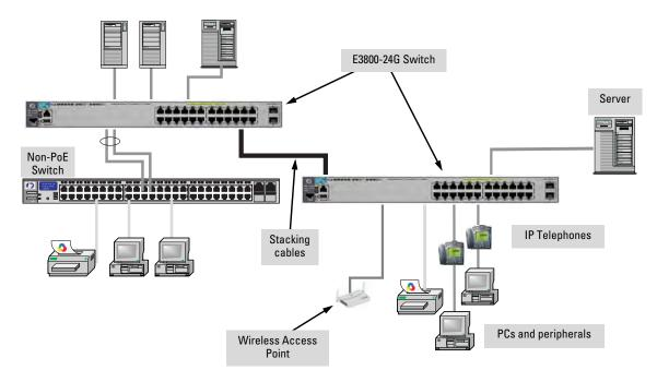
As shown in Figure 2-20, the IP telephones have been inserted in between the E3800-PoE+ switch and the PCs, and a WAP has been connected to the E3800-PoE+ switch. Only devices directly connected to the PoE+ switches can receive PoE/PoE+ power. Devices connected to a non-PoE+ switch cannot receive PoE/PoE+ power.
