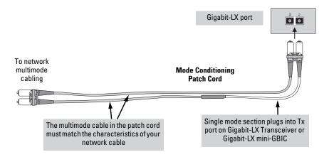
Make sure you purchase a patch cord that has appropriate connectors on each end, and has multimode fibers that match the characteristics of the multimode fiber in your network. Most important, the core diameter of the multimode patch cord must match the core diameter of the multimode cable infrastructure (either 50 or 62.5 microns).
