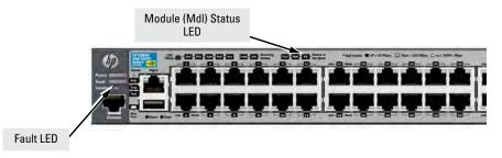
If the module is installed properly and the switch is powered on, the module undergoes a self test that takes a few seconds. You can use the LEDs to determine that the module is installed properly and has passed the self test, as described in the "LED Behavior" table below.
