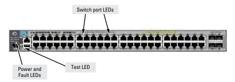
When the switch is powered on, it performs its diagnostic self test and initialization. This boot process takes approximately 50 seconds to complete.
