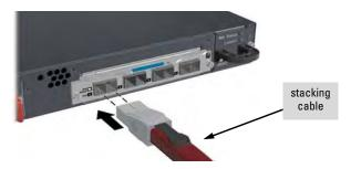
**b.** Connect the other end of the cable to a Stacking Module in another E3800 switch. See page 2-23 for connectivity.
