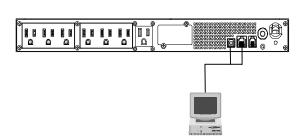
Install PowerPanel® Business Edition software on the primary computer connected to UPS with either a serial cable or USB cable.
