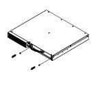
1. Remove two screws and right side front panel
