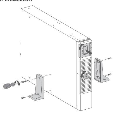
Note: The two supports for the tower position are used on the RT 2U version only.
