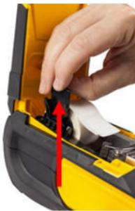
5. If you do not want to load any more media, close the printer cover by pressing down on the cover until it catches.
