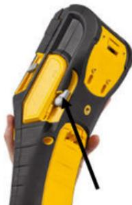
3. If label spool is not empty, gently rewind the spool with your finger to back the unused media out from under the print head.
