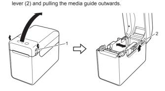
Insert the RD Roll so that the labels feed with the side to be printed on facing up (1), as shown.
