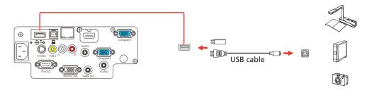
If you connect a digital camera, USB flash drive, or USB storage device, you can use the projector's PC Free feature. You can also connect other Epson document cameras to the projector. See the online *User's Guide* for details.
