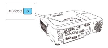
**Note:** To shut down the projector, press the power button twice, then unplug it. You don't have to wait for the projector to cool down.
