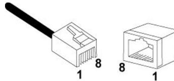
Figure 30. RJ-45 Connector and Port Pin Layout
