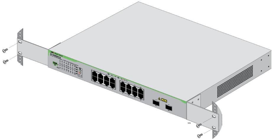
Figure 22. Mounting the Switch in an Equipment Rack
