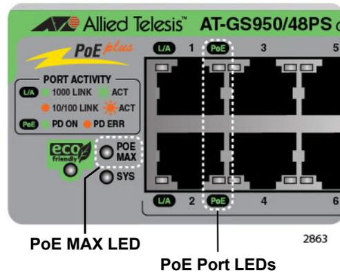
Figure 16. AT-GS950/48PS PoE and PoE MAX LEDs
