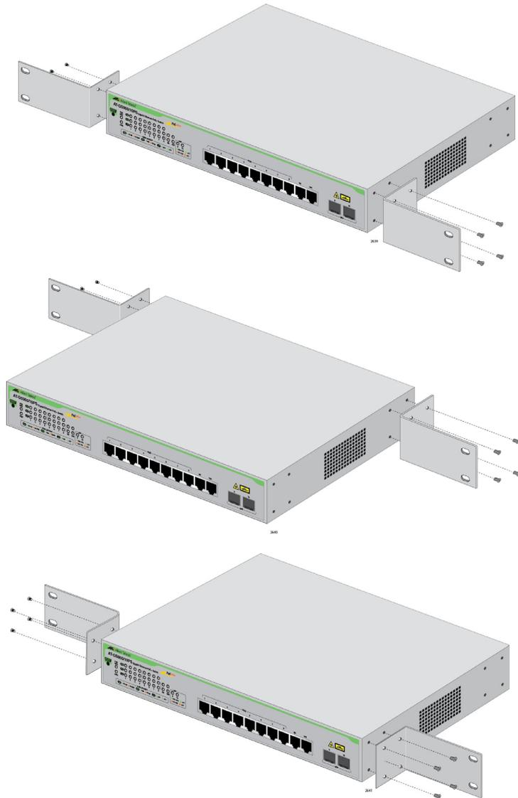
Figure 20. Attaching the Rack-Mount Brackets to the Switch
