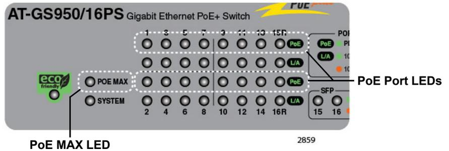
Figure 15. AT-GS950/16PS PoE and PoE MAX LEDs
