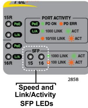
Figure 12. AT-GS950/16PS SFP Status LEDs
