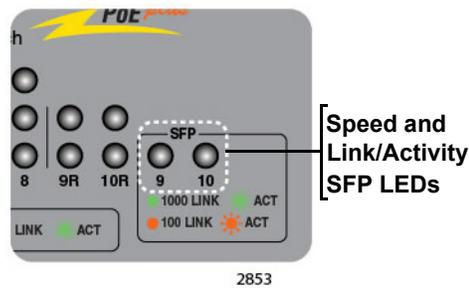
Figure 11. AT-GS950/10PS SFP Speed and Link/Activity LEDs
