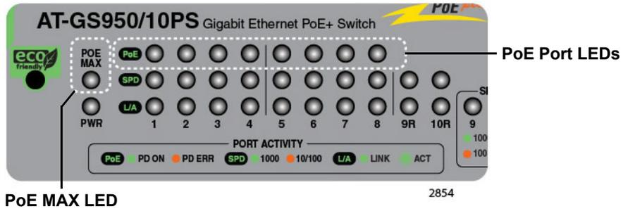
Figure 14. AT-GS950/10PS PoE and PoE MAX LEDs
