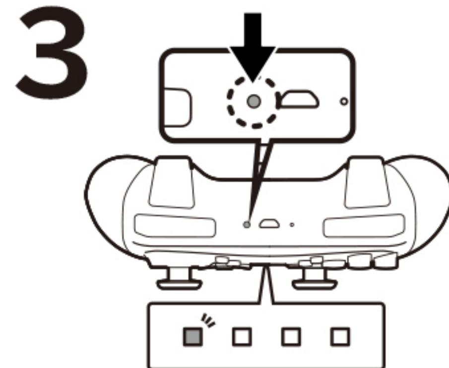
Press and hold Sync Button for at least two seconds.
