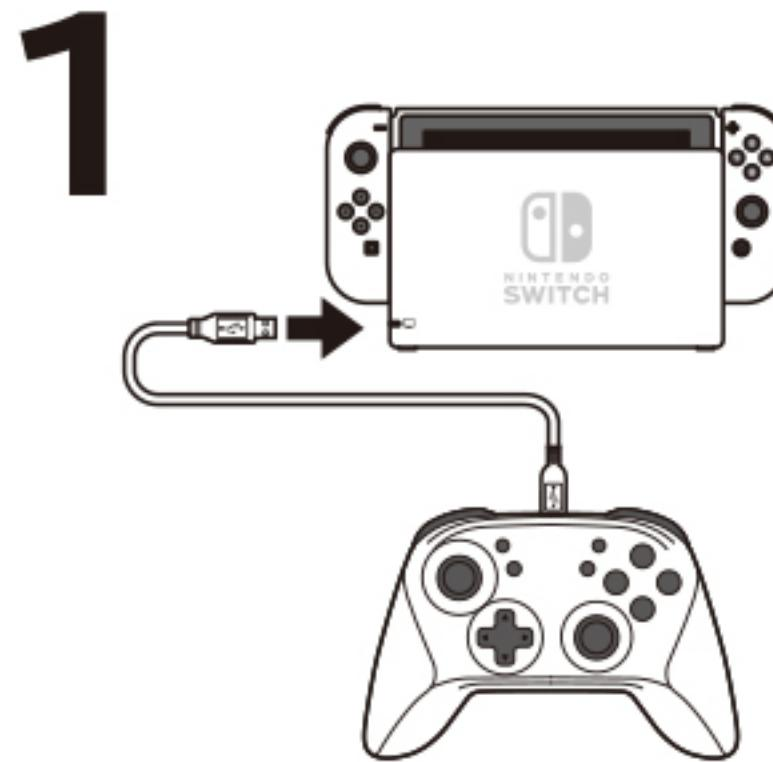
Connect using a USB-C port cable (included).
