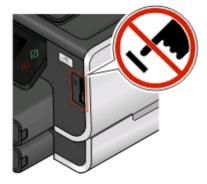
**Warning—Potential Damage:** Do not touch any cables, any network adapter, any connector, the USB Bluetooth adapter, or the printer in the areas shown while actively printing, reading, or writing from a Bluetooth-enabled device. A loss of data can occur.
