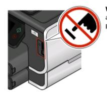
**Warning**—**Potential Damage:** Do not touch any cables, any network adapter, any connector, the memory device, or the printer in the areas shown while actively printing, reading, or writing from the memory device. A loss of data can occur.
