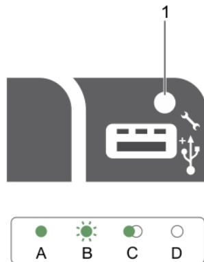
Figure 9. iDRAC Direct LED indicator
