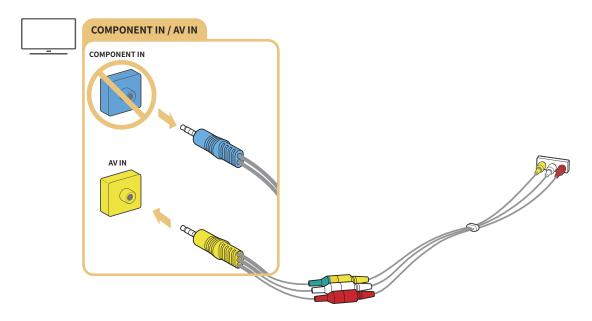
If you want to use AV (composite) equipment, remove the component adapter.
