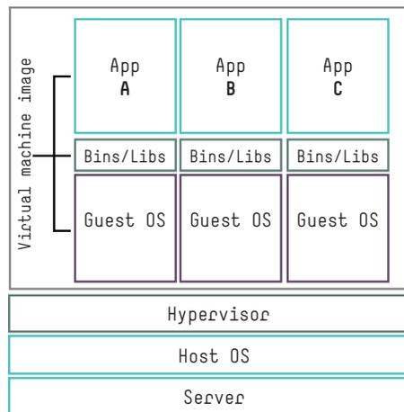
With containers, virtualization is achieved at the operating system (OS) level instead of at the hardware level like virtual machines.
