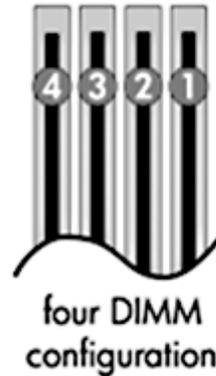
If only using 1 DIMM, install in socket 1. If using 2 DIMMs, install them in sockets 1 & 3. If using 4 DIMMs, install them in all sockets.
