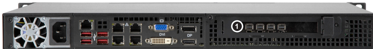
Figure 3-12. Expansion Card Chassis Slots
