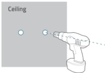
3. Align the holes on the mounting plate with those in the ceiling. Insert the anchors into the holes; anchors are necessary for walls that are made out of hard materials such as concrete, brick, or stucco. Fix the screws with a Phillips-head screwdriver to fasten the mounting plate to the ceiling.
