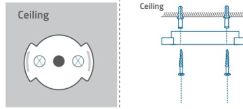
4. Align the grooves with the mounting plate and rotate the Indoor Cam clockwise until it clicks into place.
