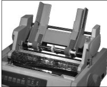
Installing the cut sheet feeder
