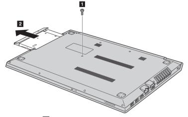
6 Remove the screw 3, then remove the removable module bracket in the direction shown by arrow 4.
