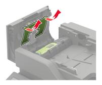
4 Remove the used ADF feed roller.
