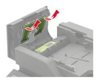
4 Remove the used ADF pick roller.
